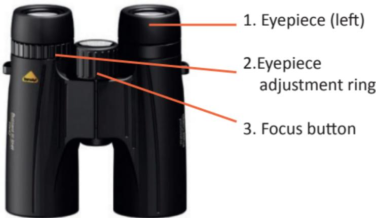
The first setting is on the left eyepiece\*\* (1). Point the binoculars to an object approx. 100 meters from where you are. While looking through the left eyepiece, cover the right barrel with your hand to prevent distraction. Now focus on the object, using the central focus button
