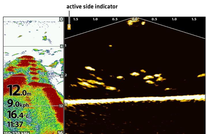
The MEGA Live/2D Zoom Combo View shows sonar information and MEGA Live Imaging information in a combination split screen, where the 2D Sonar View is displayed on the right and the MEGA Live View is displayed on the left.
