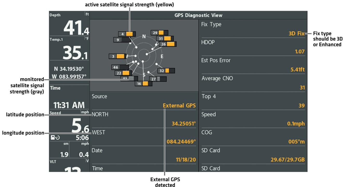
**GPS Reception:** The sky chart displays the satellite number and signal strength bar.
