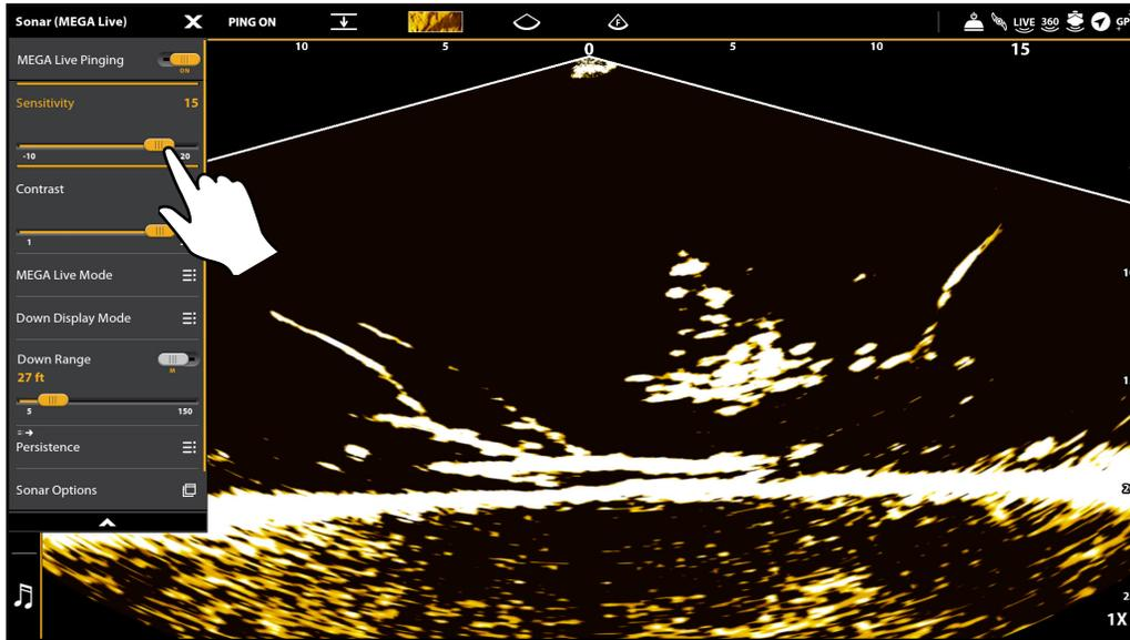
**NOTE:** The Sensitivity and Contrast are set high in the above illustration. The high Sensitivity setting displays more weak returns on the display, and the high Contrast setting shows more definition between the light and dark returns.
